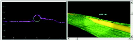
Example of CrossProfile and Virtual 3D Displays of a Pipeentering aRockdump
