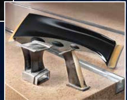
Composite parts used in aerospace applications, where porosity and voids can have catastrophic consequences
